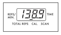
continuous display, repeatedly press the mode button. The mode indicators will show which mode is selected. (Make sure that the scan mode is not selected.)
